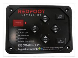
If you attempt to extend individual jacks by pressing the Down Keypad buttons or all the jacks with the Auto-Level button, you will hear a "deny" tone from the keypad if the ignition key is in the improper position.
