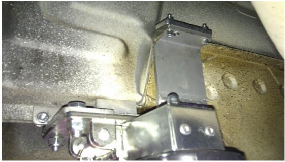
Put the adapter most front possible, if necessary remove any sealing material for a perferct adherence, use a bottle jack to stop the bracket in the correct position and make the 8mm side hole then fix with the bolt.
