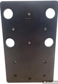
Location: Using the mount plate as a template, mark, and drill four 10mm holes at the chassis extension point as shown. The mounting plate is designed to mount over the outside of the chassis four extension bolts.
