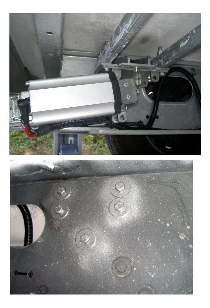
Rear Mounting Plate for Alko (HIGH) Chassis Part No. TI-0531-P-0021
