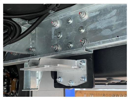
Install the two cross braces supplied on the top of the jack bracing bracket as shown using the four longer 10mm bolts.
