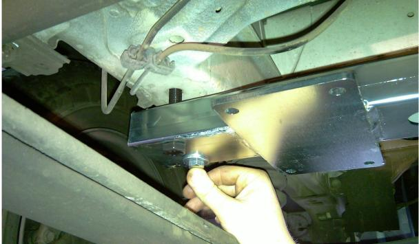
Insert and position the sealing plate (plate with **ONE HOLE**) then fix with the bolts (10x70 and 14x70).
