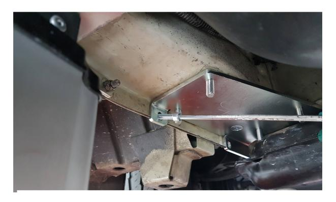
Fix with the 2 M8 bolts supplyed
