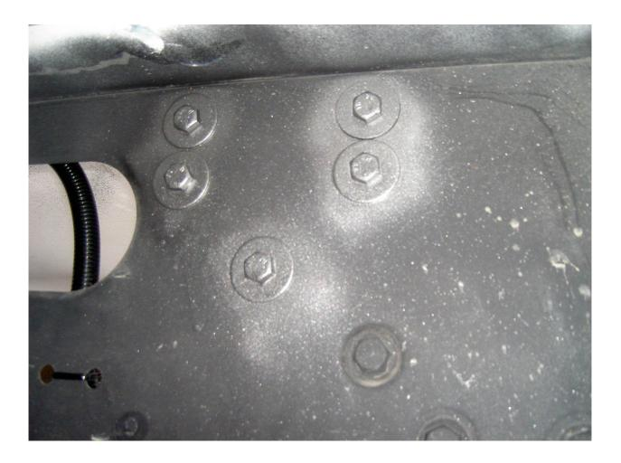
Rear Mounting Plate for Alko (HIGH) Chassis Part No. TI-0531-P-0021
