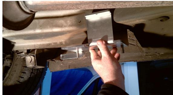
Put the adapter most rear possible, if necessary remove any sealing material for a perferct adherence, use a bottle jack to stop the bracket in the correct position and make the 8mm side hole then fix with the bolt.
