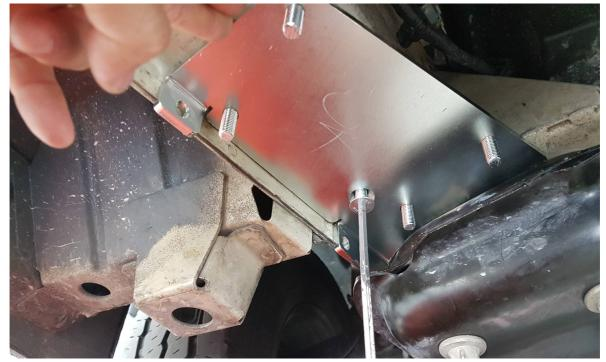
Fix the adapter with the special plate that you insert in the hole
