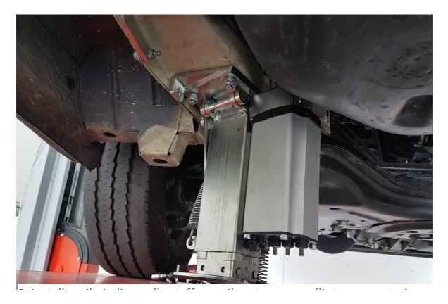
If necessary loose the bolts of the support of the tank and move it a few centimeter inside the vehicle
