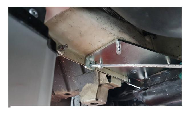
Fix with the 2 M8 bolts supplyed
