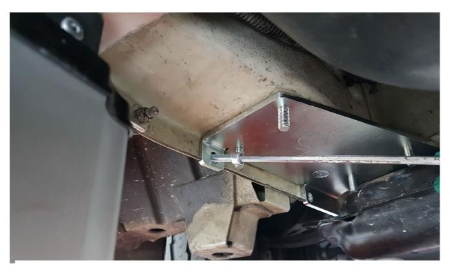
Fix with the 2 M8 bolts supplyed
