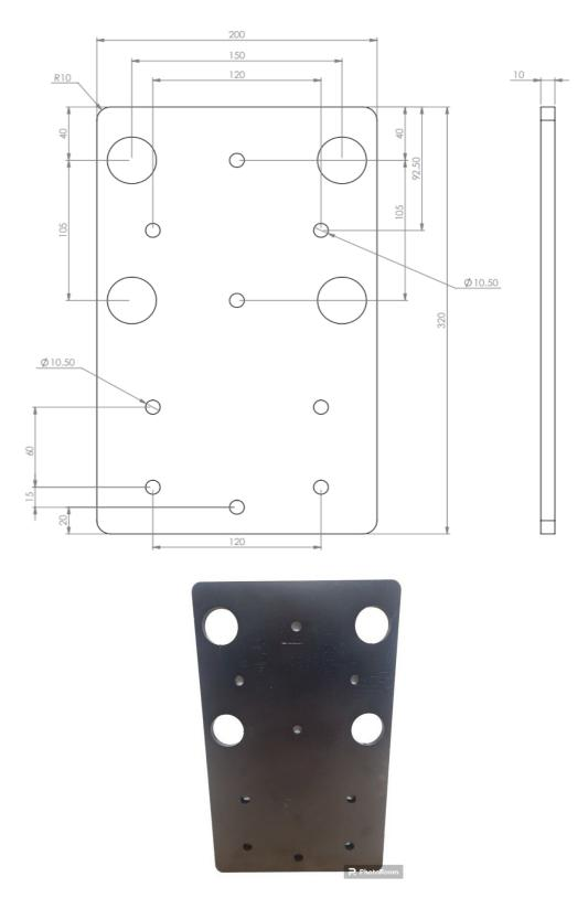
Location: Using the mount plate as a template, mark and drill four 10mm holes at the chassis extension point as shown. The mounting plate is design to mount over the outside of the chassis four extension bolts.
