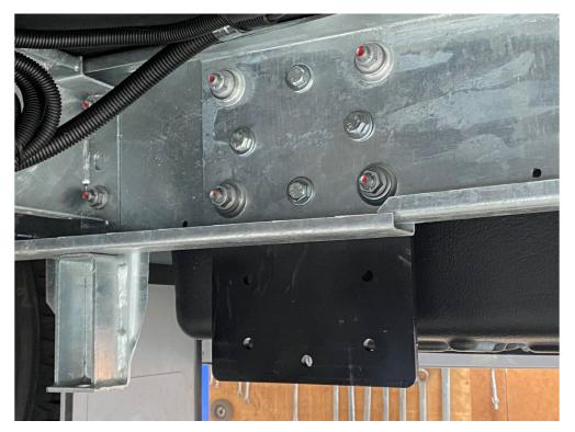
Install the jack bracing bracket by using the five 10mm bolts/nuts supplied as shown below.
