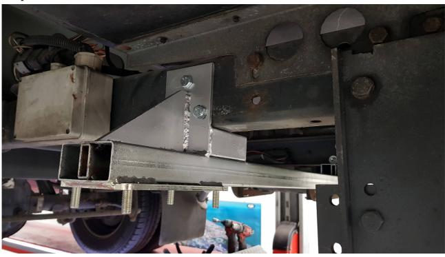
Put the adapter rear the rear axle, be carefull that the adapter is completely insert before drill the holes, is some case is possible to use holes already present on the chassis.
