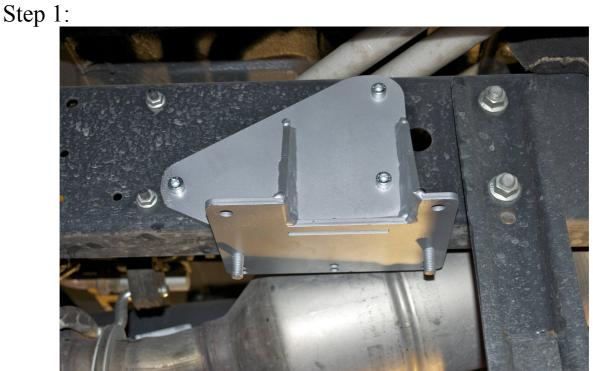
The adapter must be placed just behind the gearbox cradle, follow the same procedure as the front left adapter
