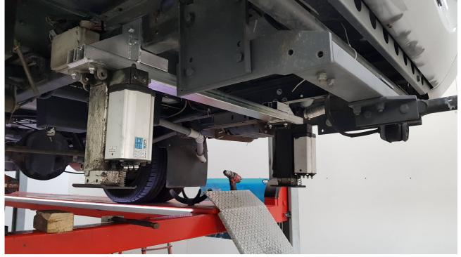
EXAMPLE OF INSTALLATION OF FRONT JACKS ON IVECO
