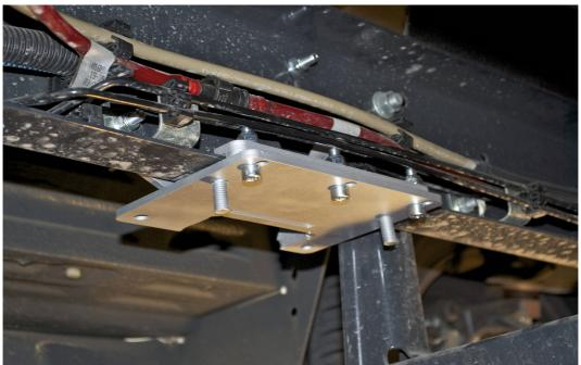
Then mount the clamp on the inside of the frame.
