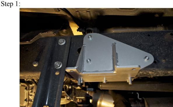
The adapter must be placed just behind the gearbox cradle and is fixed using the three M8 screws supplied, without drilling any holes on the frame if the frame is of the latest model (BLACK) otherwise drill the 3 holes.
