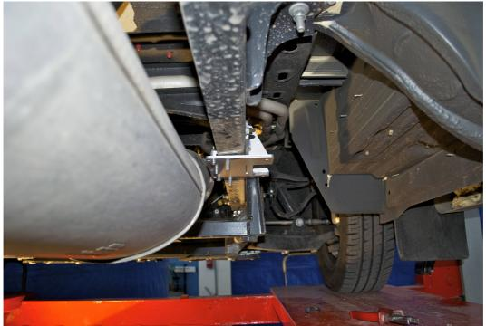
Then mount the clamp on the inside of the frame.
