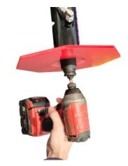
Step 2. Use an impact wrench to secure nut or bolt in place.
