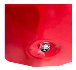
Step 3. Check the rod thread is exposed once the nyloc nut is tightened. For nylock bolt make sure it is recessed into the foot plate. The foot plate is secured with minimal movement on extensions and no movement when retracted.
