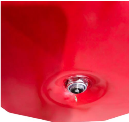
Step 3. Check the rod thread is exposed once the nylock nut is tightened. For nylock bolt make sure it is recessed into the foot plate. The foot plate is secured with minimal movement on extensions and no movement when retracted.
