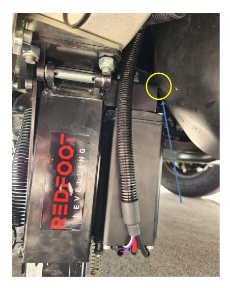
To relocate the tank towards the driver's side, drill two new holes in the existing tank straps.
