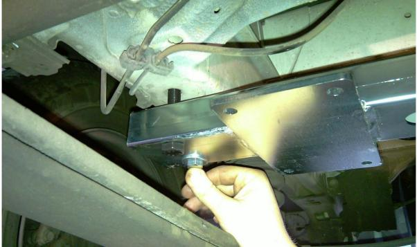
Insert and position the sealing plate (plate with **ONE HOLE**) then fix with the bolts (10x70 and 14x70).
