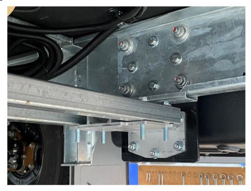
Install the jack leg into position as shown and tighten the bolts/nuts. Ensure washers are also used.
