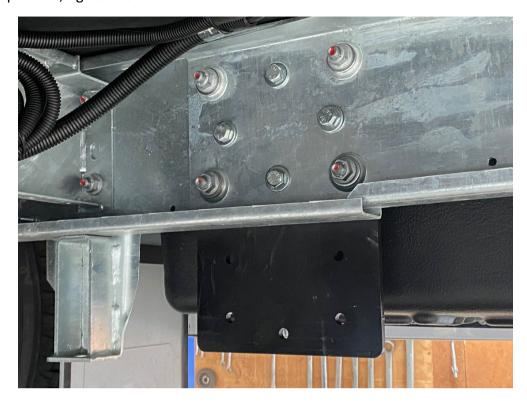
Install the jack bracing bracket by using the five 10mm bolts/nuts supplied as shown below.
