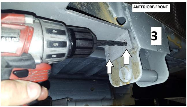
Step 3: Push the adapter on the frame then drill two 10mm hole and fixs with the bolts supplied.
