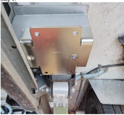
Put the adapter in the point illustrated (rear the rear axle), drill one 10mm hole at the internal side of adapter then insert the special plates and fix the adapter with the M10 bolts supplied
