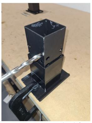
Step 3. DRILLING THE PIN HOLES - Clamp the foot firmly to the bench and using a 9mm drill bit, drill out the two holes (do this to the holes on opposing sides sides). This helps to insert and align each of the pins.
