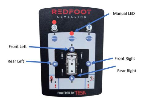
To set limit switches you will need to press the manual button and a selected jack arrow button at the same time, this will operate and extend the jack until it reaches the vertical position. The system answers with consistent beeps and the selected jack light will flash. To retract the jack to the stowed position, press the jack arrow button.
