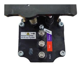
After fitting (purple cable only) make sure to fill the rubber cap with the supplied grease. Do not grease or fit rubber cap before securing cables to avoid grease affecting contact with the post. The grease avoids accidental ground with other connections caused by splashes of water and/or debris.
