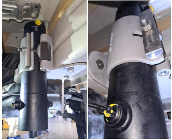
Adjust the cylinder to correct height from the ground and tighten Nyloc nut at 50Nm using a Torque Wrench
