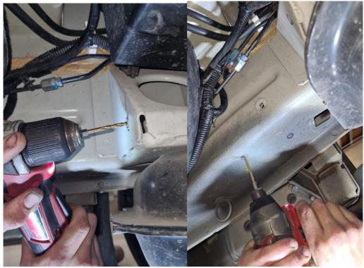
Insert Rivsert Paddle Stick inside chassis and position the bracket so the holes align. Hold the bracket into position and insert the two M10 30mm bolts into the underside of chassis, then tighten. Insert the countersunk M10 25mm Socket Head Screw bolt into the chassis side wall, ensure to use the M10 Nyloc Nut and washer, tighten using a 6mm Allen key.
