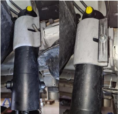
Adjust the cylinder to correct height from the ground and tighten the M10 Nyloc nut to 50Nm
