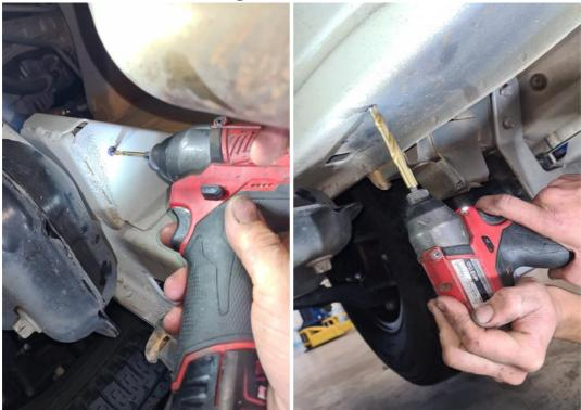
Insert Rivsert Paddle Stick inside chassis and position the bracket so the holes align. Hold bracket into position and insert the 2x M10 60mm bolts into the underside of chassis, then tighten. Insert the countersunk M10 25mm hex head bolt into the chassis side wall, ensure to use the washer/Nyloc Nut to tighten using a 6mm Allen key
