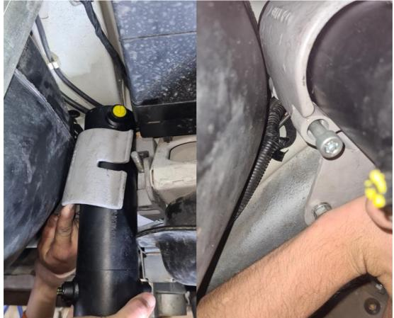
Tighten the M10 100mm Socket Head Screw bolt at 30Nm with Torque wrench.
