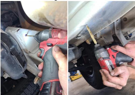
Insert Rivsert Paddle Stick inside chassis and position the bracket so the holes align. Hold bracket into position and insert the 2x M10 30mm bolts into the underside of chassis, then tighten. Insert the countersunk M10 25mm hex head bolt into the chassis side wall,
