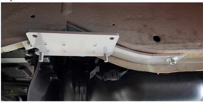
Fit the adapter with the bolts supplied
