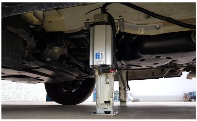
EXAMPLES OF JACKS CORRECTLY INSTALLED
