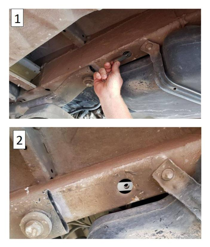
Step 1: Insert the special plate in the hole present on the frame, put the adapter and push frontly.
