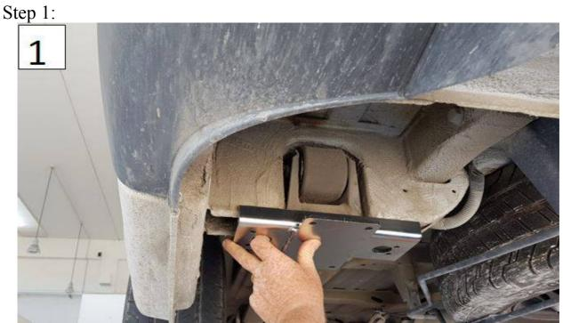
Put the adapter in the point illustrated, the rear support of the crossbow suspension
