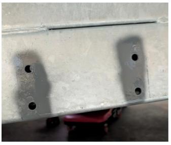
Use wax and grease remover to clean the area and holes then apply an anticorrosion paint like a cold galvanizing compound to prevent rust.
