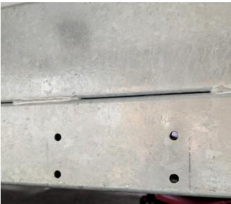
Step up your drill bit until you reach 11mm. As you can see here there is wires running through the chassis that need to be avoided.
