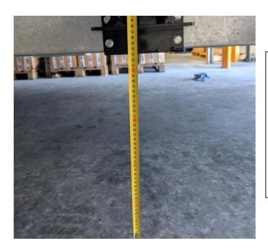
Next, measure the distance from the mounting plate of the bracket to the ground. The van chassis will need to be as level as possible, see Autolift install manual for how to add spacers to expand the jack. If you are using optional under chassis bracket spacers as shown, install them using washers provided.
