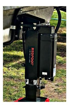
Each bracket is designed to be attached around the RHS chassis rails for these sizes. H 100mm x W 50mm - H 125mm x W 50mm - H 150mm x W 50mm
