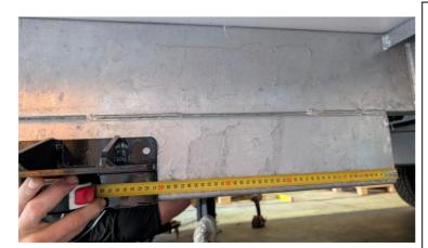
Once you have found the optimal location along the chassis rail, prior to installing make note of any obstructions. Further, consider the swing of the jack once installed, handbrake wires and suspension mounts.
