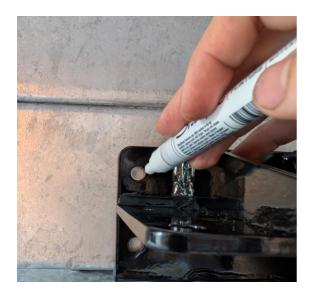
Once suitable mounting locations are found, mark where each hole will need to be drilled with the bracket flush up against the bottom of the chassis.
