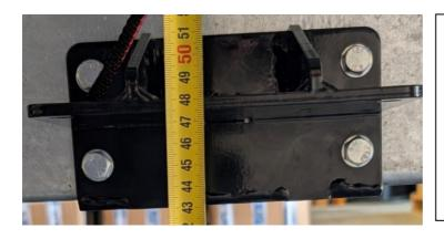
You may need to use a small screwdriver to lift the wires inside the chassis to get the bolts to slide through. Ensure you use washers with each bolt, unless the bolt interferes with the spring on the jack.
