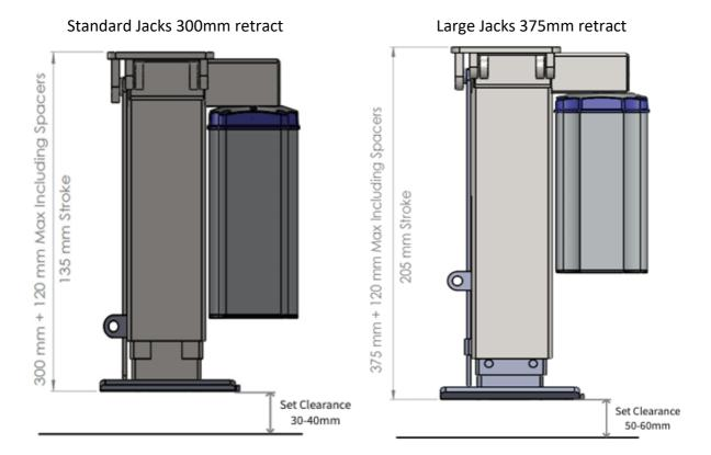
In each kit you will receive 10mm, 20mm and 40mm spacers to expand the jack up to 120mm in additional length. The spacers have been designed to allow you to achieve the desired set point once the jacks are mounted to the brackets bolted to the chassis.
