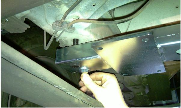
MOUNT BOTH REAR JACKS WITH MOTOR TO THE INSIDE OF THE VEHICLE AND ROTATION TO THE FRONT
