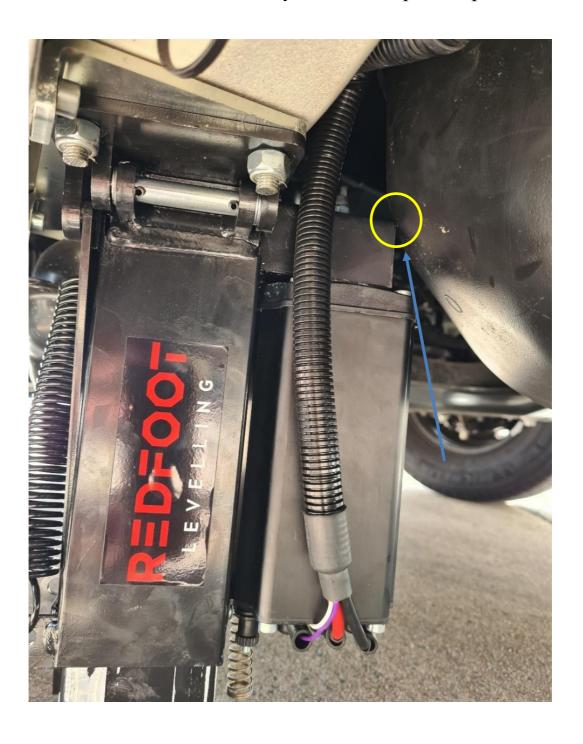
To relocate the tank towards the driver's side, drill two new holes in the existing tank straps.
