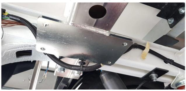
Step 2: Fix the adapter using the bolts supplied (4pc - 10x70), then fix the jacks.
