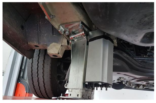
The above image shows the jack with the motor to the inside of the vehicle and rotated to the rear.
