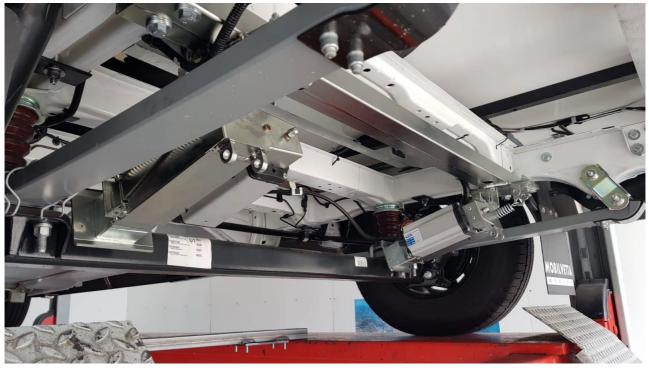
MOUNT BOTH REAR JACKS WITH MOTOR TO THE INSIDE OF THE VEHICLE AND ROTATION IN FRONT OR REAR
