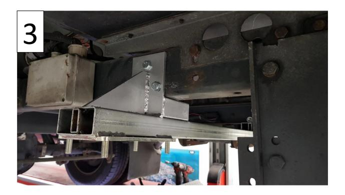
Step 3: Put the rear bracket behind the rear axle on the main chassis, make sure the bracket is pushing all the way up against the chassis before marking out the holes. On some chassis it is possible to use pre-existing holes if not drill 3 10.5mm holes on each side.
