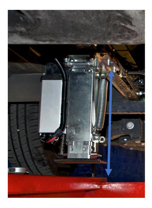
There needs to be a minimum from bottom of chassis to ground clearance of 430mm, otherwise front the suspension will need to be adjusted to reach this height.
