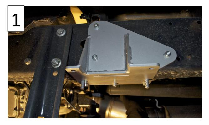
Step 1: The adapter must be placed just behind the gearbox cradle and is fixed using the three M8 screws supplied, the new models will line up without drilling any holes otherwise mark and drill 3 holes.
