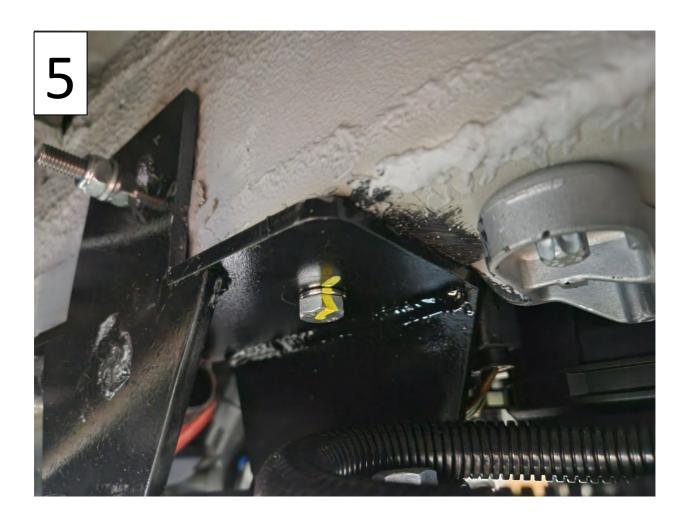
Step 5: Screw the M10 x 30mm into the nut plate to fix the bracket into place then use the M10 x 120mm bolt for the top bracket mount. Torque these to 30NM.
