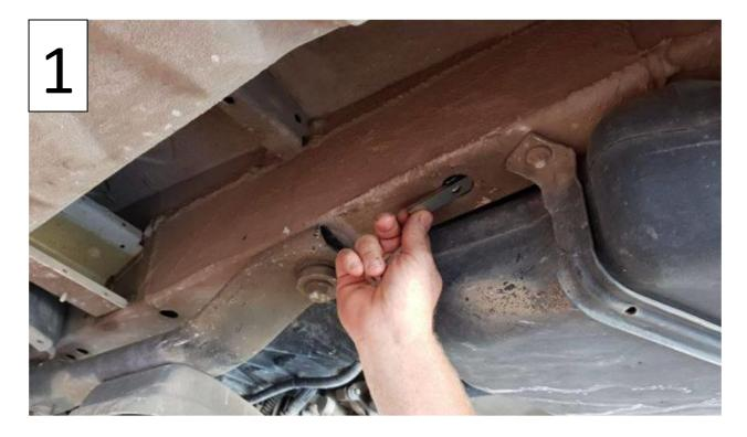
Step 1 - 2: Insert the nut plate in the hole present on the frame behind the front subframe.
