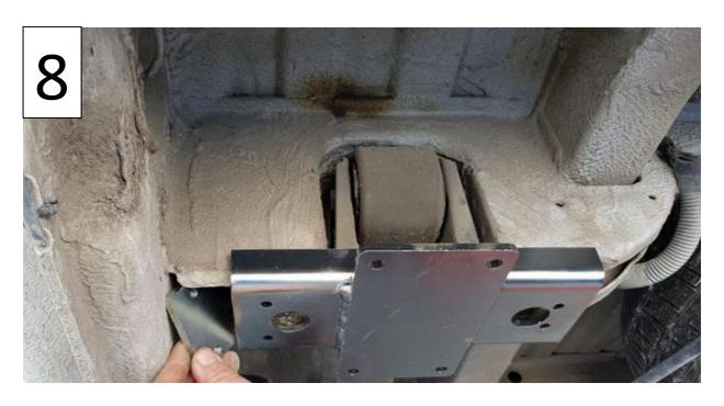
Step 8 - 9: Once both nut plates are in place use the M8 bolts supplied to fix the bracket in place. Torque these to 20NM. Repeat this for both sides of the vehicle.
