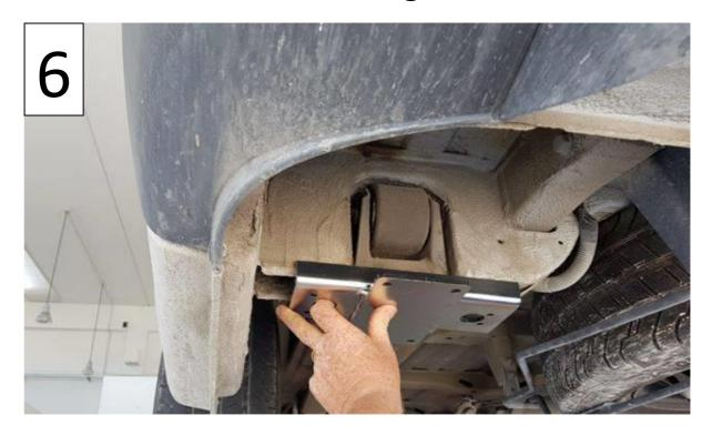
Step 6 - 7: Place the rear bracket over the spring hanger mount as shown, place both nut plates in either side of the hanger.
