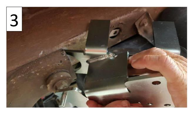
Step 3 – 4: Push the bracket firmly around the subframe mount then mark out and drill an 11mm hole into the chassis for the brackets top bolt.
