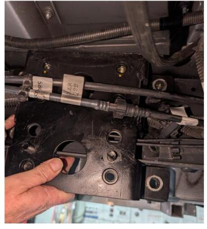
Hold into place and insert the flange bolts and nuts as required.
