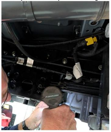
Place the cylinder onto mounting bracket.
