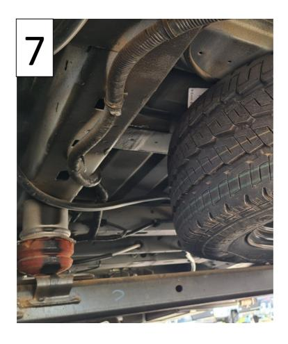
Step 7 - 8: Move any wires out of the way and place the rear bracket along the chassis behind the bump stop as shown, a new 10.5mm hole may need to be drilled.
