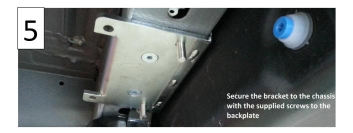
Step 5: Secure the bracket to the chassis with the counter sunk screws supplied into the nut plate. Torque these to 20NM.
