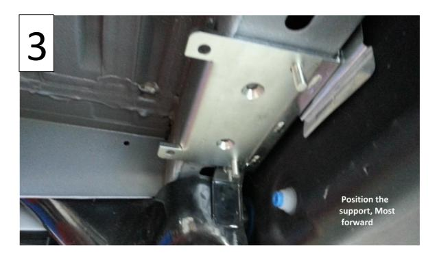
Step 3: Place the bracket as far forwad as possible then mark out and drill the two holes to 10.5mm.
