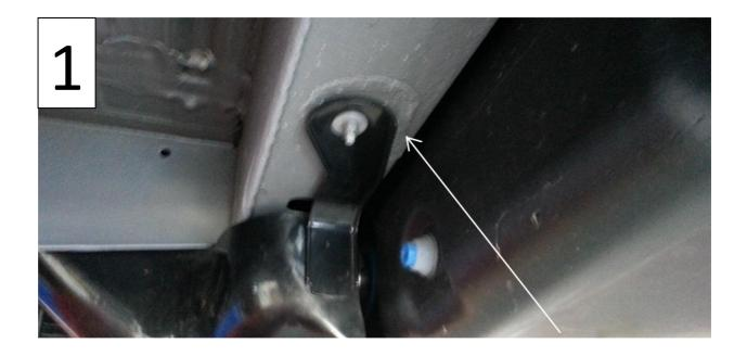
Step 1 - 2: Locate fuel filler hose bracket and modify as shown and reconnect using an M6 bolt and nut. Cut and grind off the threaded stud so there is a flat surface.
